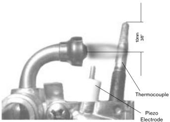
Fig. 7 - Characteristic Pilot Flame
